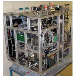
Figure 3: Technology Platform 2: Fuel cell APU laboratory prototype during assembly.
